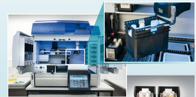
EasyKit reagent sets can be used directly in the device-specific mounts of the fully automated machine Agility®. A 2D barcode with lot-specific test information ensures safe management of the reagents.
